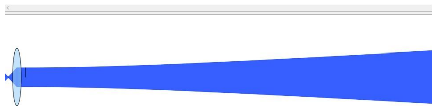
Fig. 8: Laser source at the focal point of lens [66]
