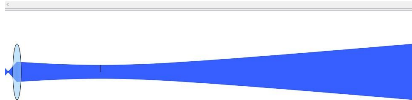
Fig. 12: Maximum achievable output beam waist position [66]
